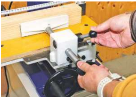
▲ A push in clamp, locked with the cam lever secures work firmly
